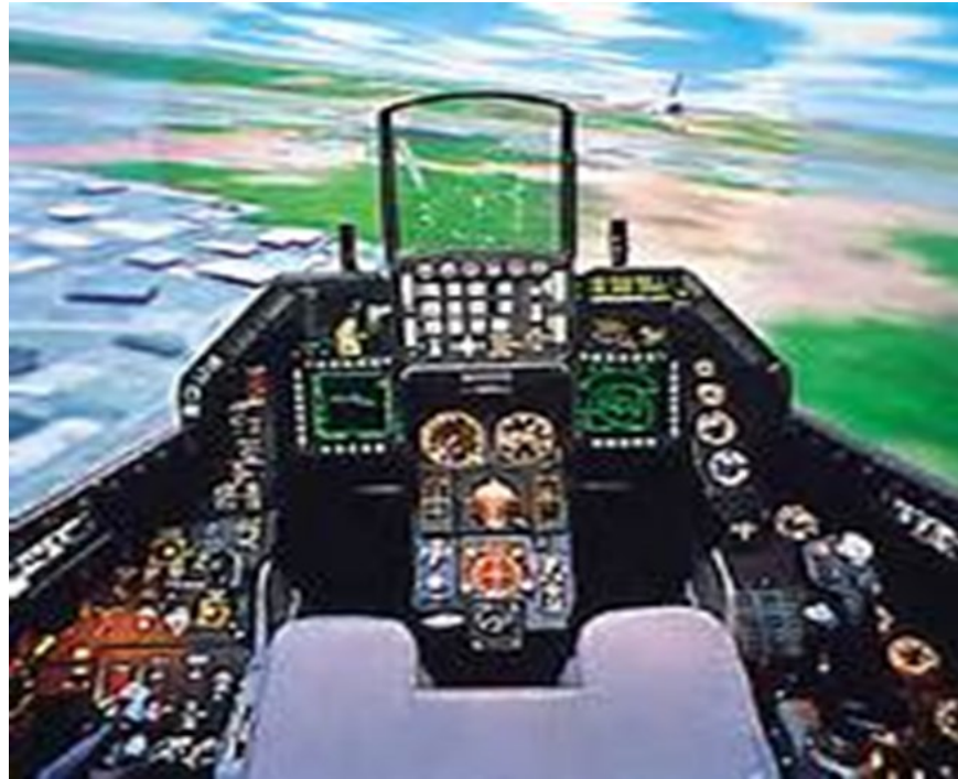
Figure 15. A simulator cockpit with a high level of simulation fidelity in the cockpit and a medium level of fidelity in the outside visual scene.
