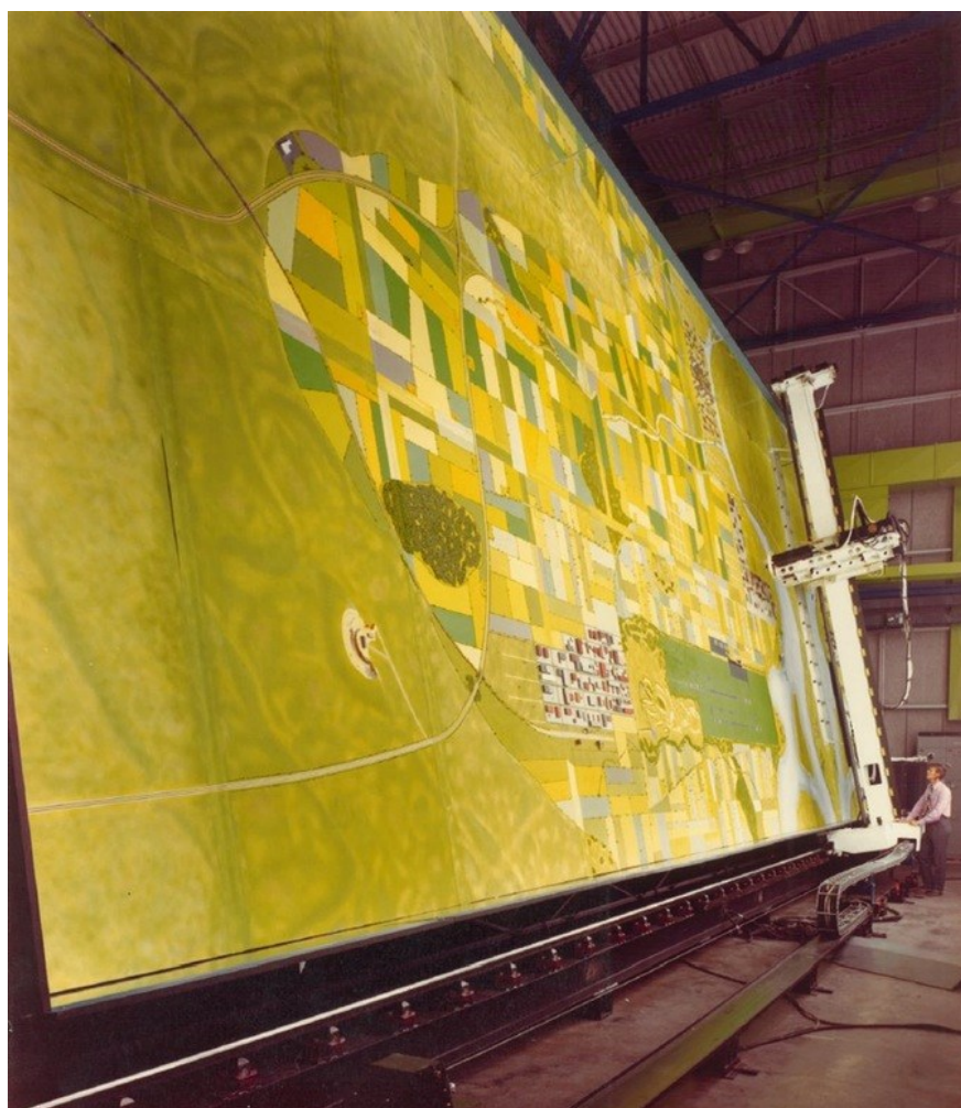
Figure 17. 3-D Terrain board for flight simulation visual scenes
